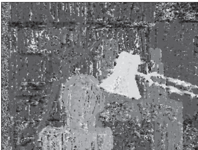
Figure 1: Disparity Depth Map resulting from naïve belief propagation algorithm for 5000 iterations
