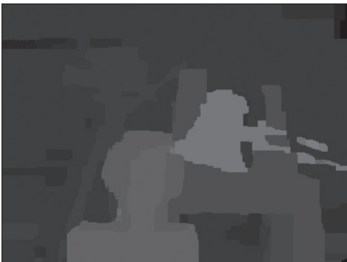
Figure 2: Disparity Depth Map resulting from naïve belief propagation algorithm with Felzenszwalboptimizations for 5000 iterations
