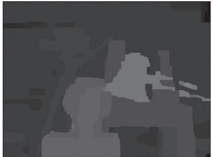
Figure 3: Disparity Depth Map resulting from Felzenszwalb belief propagation algorithm with 5000 iterations
