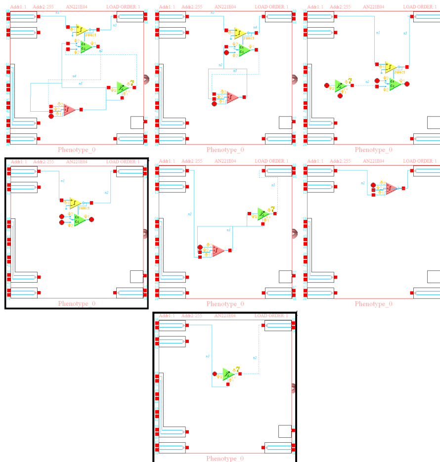
Figure 6.12: Example of champion non-specialist phenotype, showing the 7 possible circuit expressions. The first circuit shows the fully specified genome containing SumIntegrator, GainSwitch and GainVoltageControlled CAMs. This phenotype scored 2644 and deployed 2 circuits (no. 4 at 5kHz and no. 7 at 1kHz, shown with additional borders). Again note the poor but sufficient circuit deployed for the 1kHz stage.
