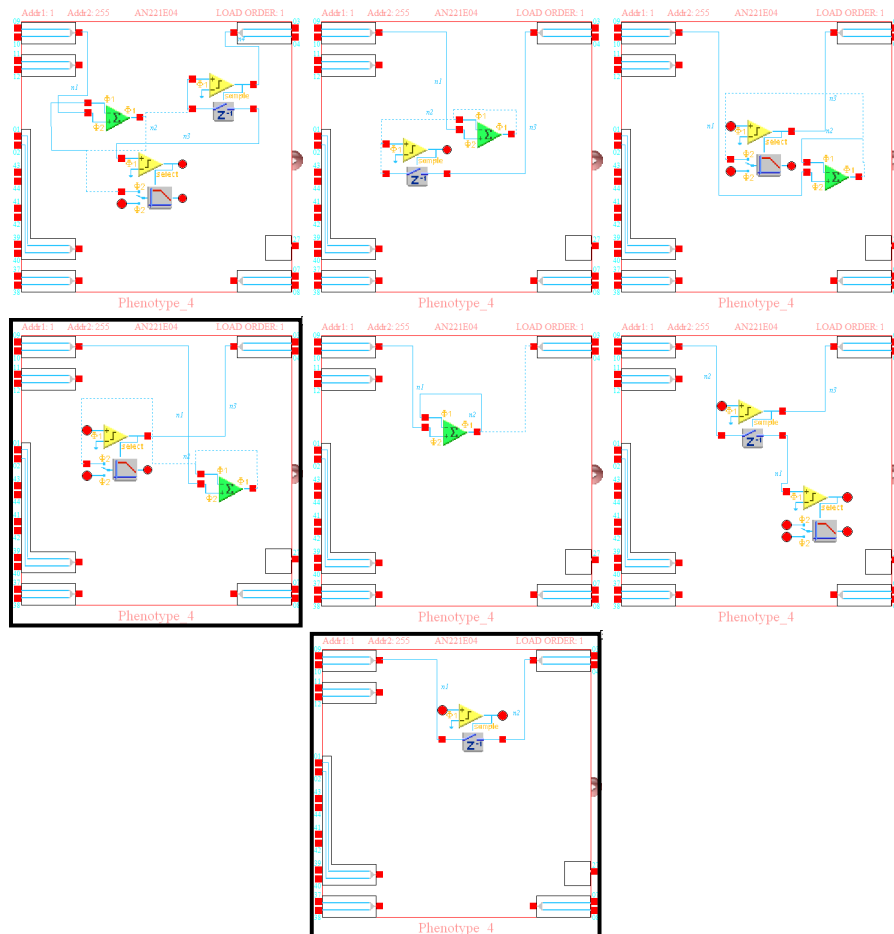
Figure B.4: Examples of champion non-specialist phenotype, showing the 7 possible circuit expressions. The first circuit shows the fully specified genome containing HoldVoltageControlled, GainSwitch and SumDiff CAMs. This phenotype scored 2670 and deployed 2 circuits (no. 4 at 1kHz and no. 7 at 5kHz, shown with additional borders). The experiment is described in §6.6.
