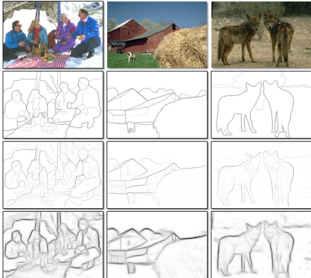
Figure 2. Illustration of edge detection results on the BSDS500 dataset: (top row) original image, (second row) ground truth, (third row) results of SCG [31], and (last row) our results for SE-MS.
