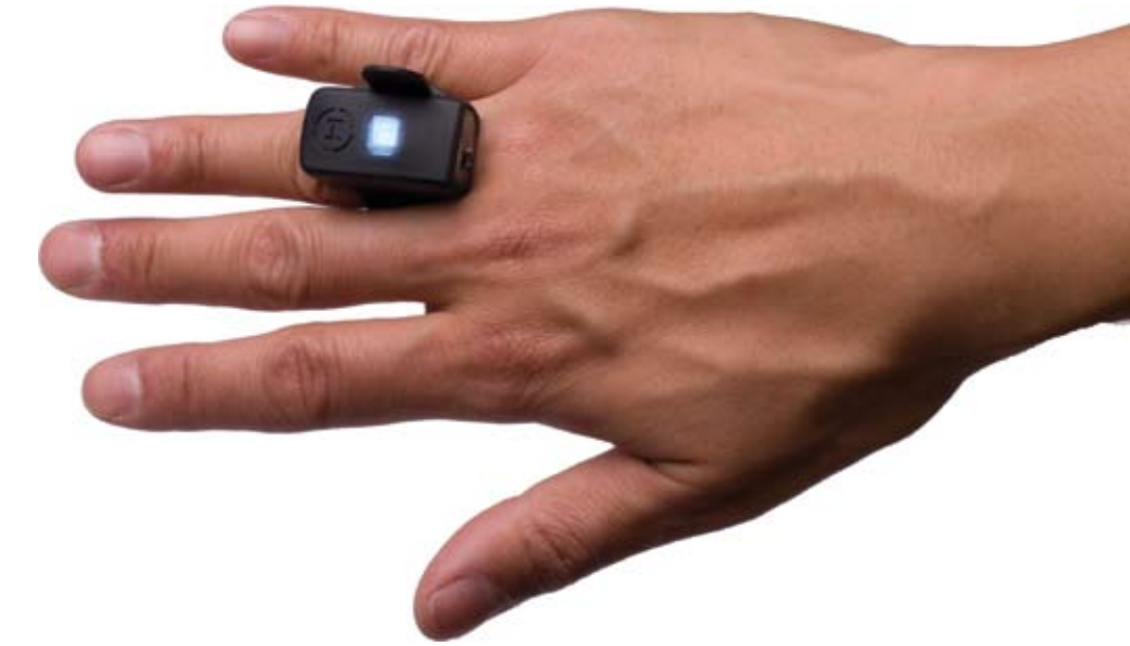
↑ The HotHand device: a ring worn by electric guitar players that uses motion sensors and a wireless transmitter to create different kinds of sound effects by various hand gestures.
