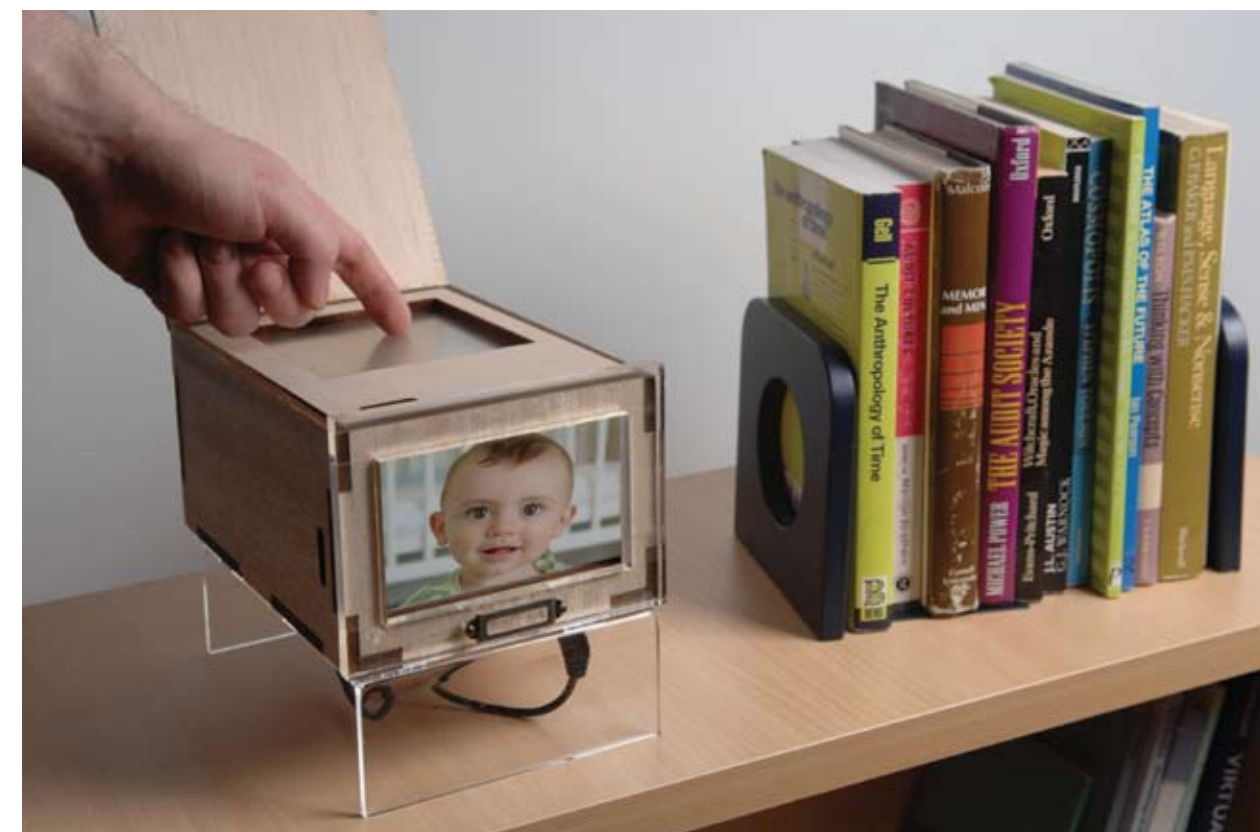
← The Digital Shoebox, by designer Richard Banks of Microsoft Research Cambridge UK, is an attempt to make the storage of digital photos more tangible. Photos can be sent wirelessly to the box, and users can browse through them by running their finger across the top of the box.
