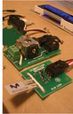
↑ Phidgets or 'physical widgets' are building blocks to help developers construct physical user interfaces. These arose from a research project led by Saul Greenberg at the University of Calgary.
