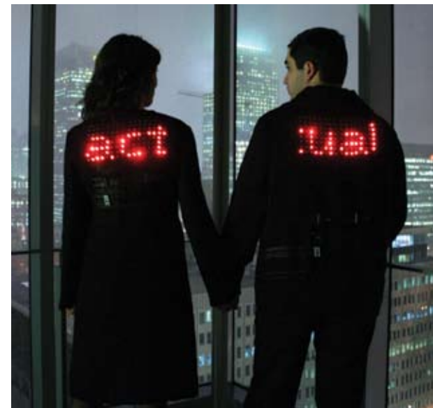
Animated Textiles developed by Studio subTela at the Hexagram Institute, Montreal, Canada. These two jackets 'synchronise' when the wearers hold hands, and the message scrolls from the back of one person to the other. →
