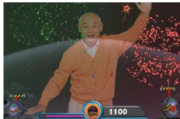
Sony's EyeToy being played by grandpa. A camera on the TV projects his image on to the playing screen, allowing him to interact with the game using arm movements and gestures. →
