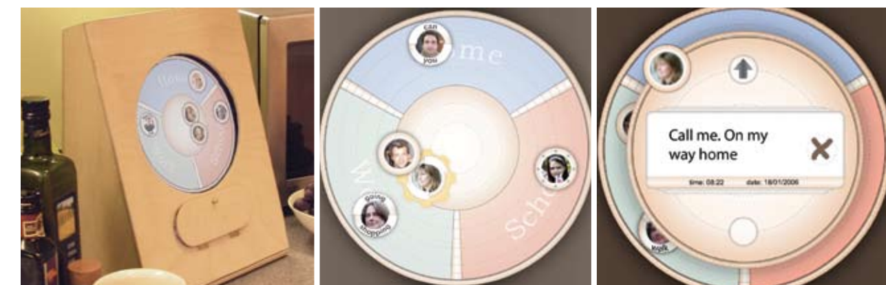
← The Whereabouts Clock: the lefthand image shows the clock in its case; the middle image is a close-up of its interface; and the righthand image shows what happens when you touch on a text message.
