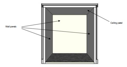
Panels will be installed on the walls and ceiling and will be composed by a sandwich of materials with fire resistance and thermal insulating to resist high temperatures and provide a watertight enclosure.
