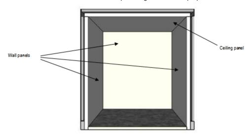
Panels will be installed on the walls and ceiling and will be composed by a sandwich of materials with fire resistance and thermal insulating to resist high temperatures and provide a watertight enclosure. The sandwich will be covered by one layer of galvanized steel sheet (0,6 mm), joined by continuous weld panel to panel.
