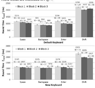
Fig. 7 Per-key round trip times for *Default* (top) vs. *New* (bottom).
