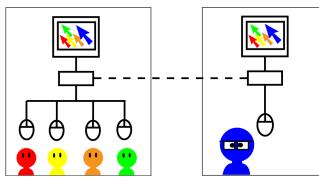
Figure 1. The Mischief system. Left: multiple, collocated students use a shared display. Each student is represented by a small colored cursor. Right: a remote instructor sees identical content on her screen and is represented by a larger cursor.
