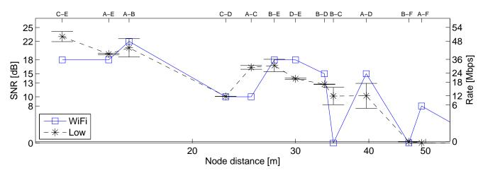
Fig. 2. The average SNR and the corresponding rates for different links in the network from Figure 1. On the top x axis we mark each link and on the bottom x-axis we plot the corresponding link lengths. On the left y-axis we plot the average SNR and on the right y-axis we plot the corresponding transmission rate, based on the measurements from [12].
