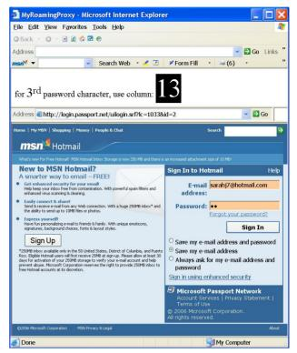
Figure 4: Sample screen capture of the proxy server interface. The upper frame tells the user which column of the table to use for the next character. The lower frame is the actual site to which the user is logging in.
