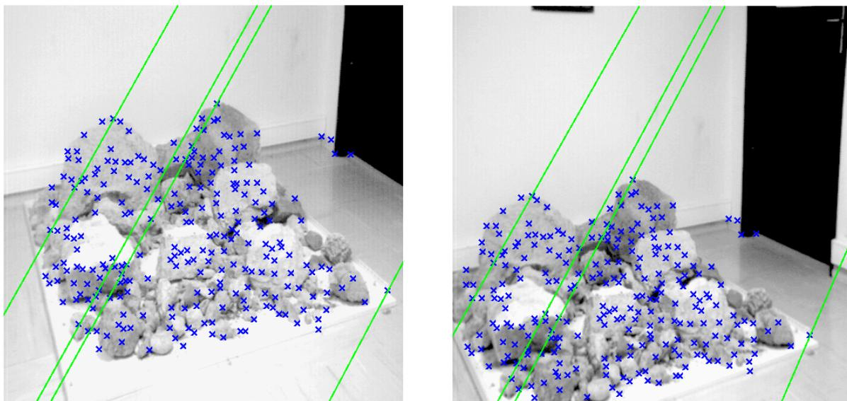
Fig. 8. Epipolar geometry estimated with the nonlinear method
