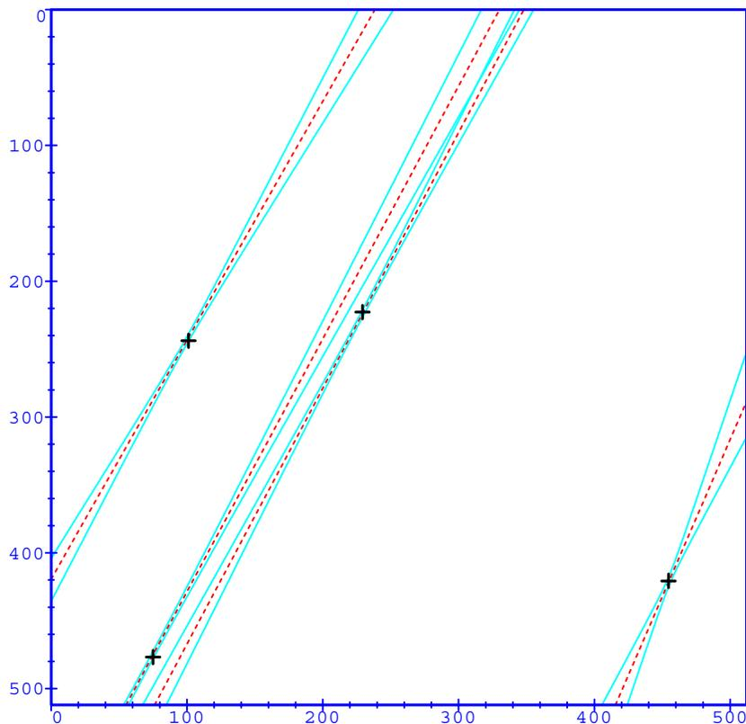
Fig. 12. Epipolar bands for several point matches
