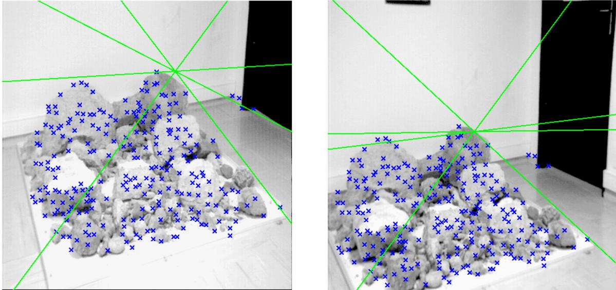
Fig. 6. Epipolar geometry estimated with the linear method
