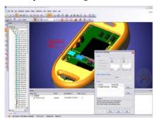
Figure 3: Combine 3D parts and ECAD designs into a single digital assembly
