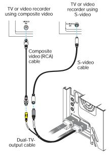
(Note: Using the Matrox composite video *and* S-video connectors at the same time is optional.)
