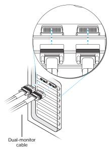
QID Low-profile PCI and PCIe – Attach your quad-monitor cable to the connector on the bracket of your Matrox card. Make sure the connectors are properly fastened.
