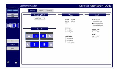
Although processed independently, the two channels are always started and stopped synchronously. The two processed inputs always include the HDMI B input and either the SDI A or HDMI A input.
