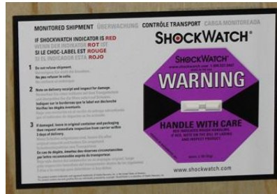
Figure 3: S530 crate shock sensor
