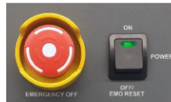
Figure 36: S530 power ON switch
