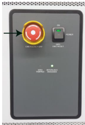
Figure 39: EMERGENCY OFF button
