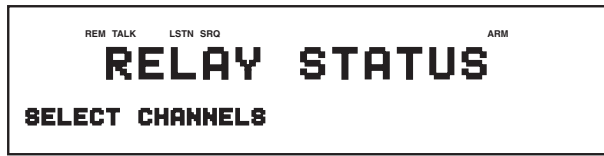
Figure 5-3 VFD relay status mode
