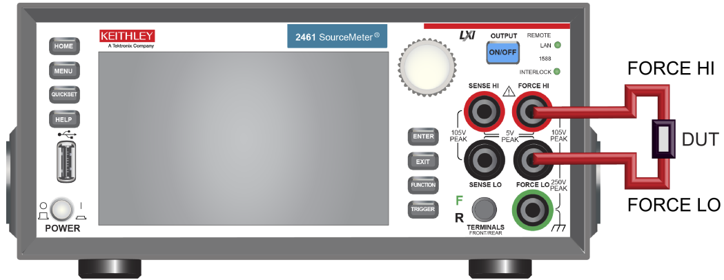
Figure 60: Model 2461 2-wire rear panel connections
