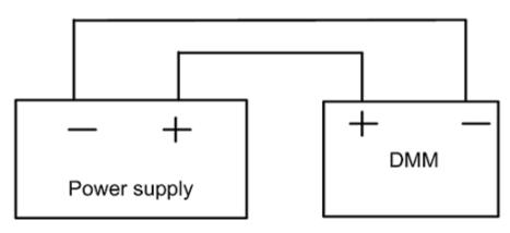
Set up the equipment for current calibration as follows.
