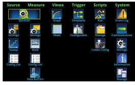
Graphical interface SMUs that utilize iconbased menu structures reduce learning curves and configuration steps, resulting in faster measurements.
