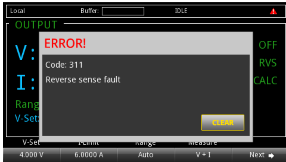
Figure 29: Reversed sense leads error
