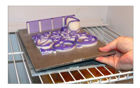
3. Within a couple of minutes, you will hear crackling sounds. This is the sound of a parts separating from the build plate.
