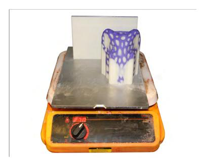
7. Within a few moments the support wax will begin to melt. Carefully touch each part(s) to see if it starts to slide across the build plate. Larger pieces will take a bit longer than smaller ones. Once all the part(s) have released, turn off the hotplate and remove each part(s) off the build plate and place on a wax paper.
