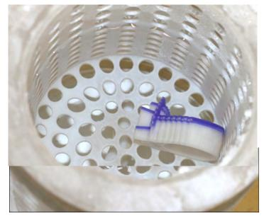
12. This part was removed from the basket after 2 minutes. You can clearly see the support material dissolving away from the build material (M3 Cast).
