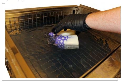
12. The below part was removed from the Ultrasonic cleaner after 3 minutes. You can clearly see the support material dissolving away from the build material (M3 Cast).
