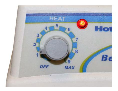
6. Fill an approved glass container with 99%> Isopropyl Alcohol (IPA) and leave at least 1" of space from the top of the container. Place on hot plate and cover with the lid to avoid evaporation.
