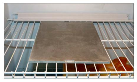
2. Place the build platform on top of the cold blank build plate as shown. Keep freezer door open.
