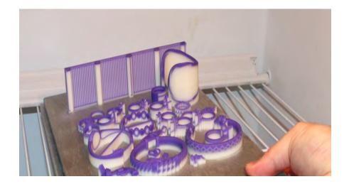
3. Within a couple of minutes, you will hear crackling sounds. This is the sound of a parts separating from the build plate. Carefully touch each part to confi rm the build part has separated from the build plate. Larger pieces will take a bit longer than smaller ones. Remove build plate from freezer when all parts have separated from build plate.
