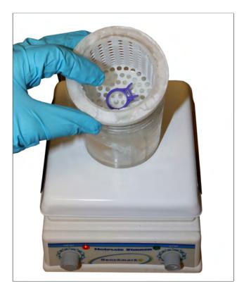
9. Turn on stirrer to a low/medium setting so that there is a nice smooth circulation in the container. If IPA is splashing out of container, turn your settings down.
