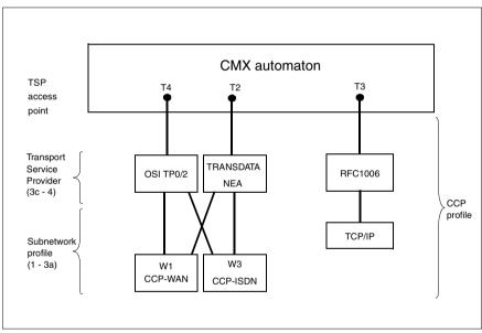
Figure 35: TSPs, subnetwork profiles, and CCP profiles
