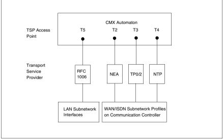
Figure 39: Logical structure of communication in UNIX systems
