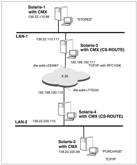
Figure 17: Sample configuration for LAN connection via X.25
