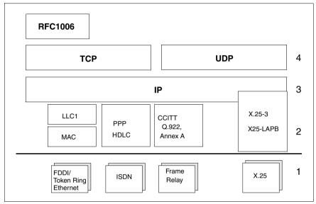
Figure 3: TCP/IP protocol stack
