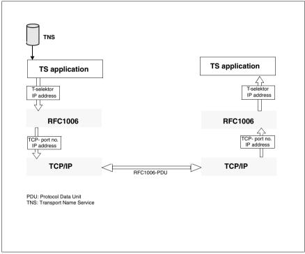
Figure 32: Connection setup via RFC1006 - overview
