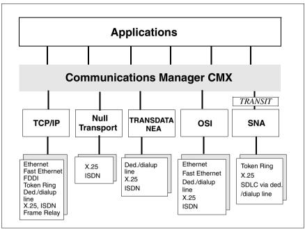
Figure 2: Network interfaces and transport profiles
