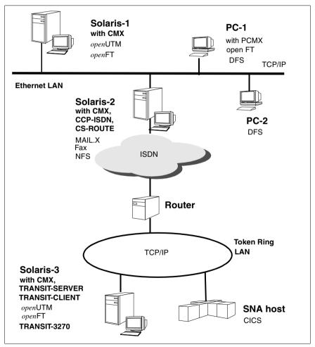
Figure 9: TCP/IP applications via ISDN
