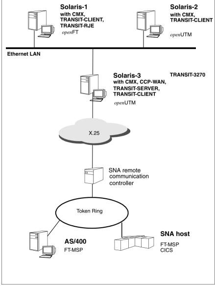
Figure 10: Connecting Solaris systems with an SNA environment
