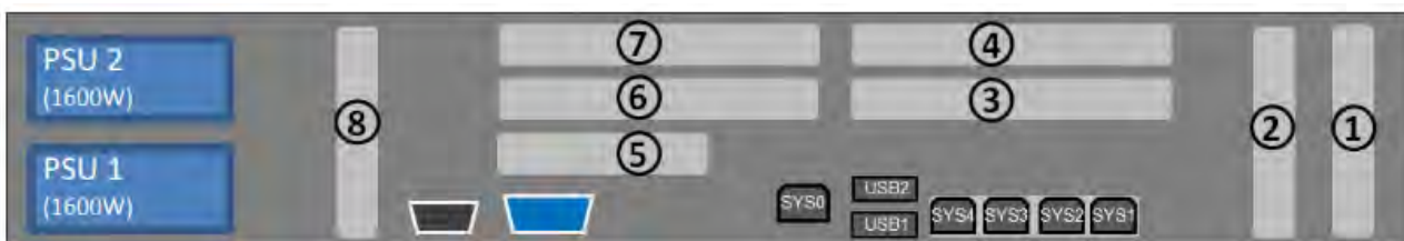
Figure 12: Principle of PCIe slot assignment at the rear of the device (SU310)
