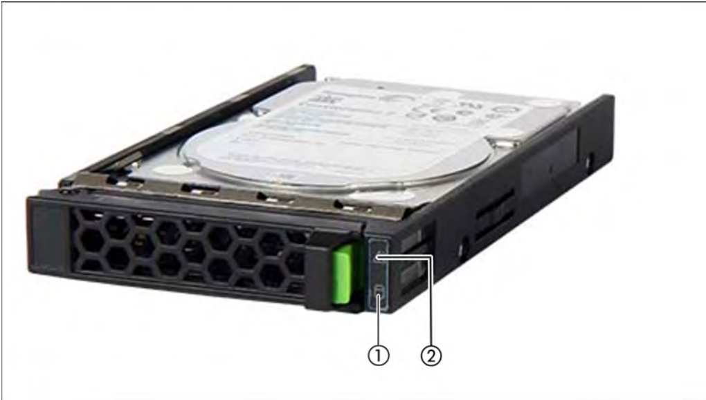
Figure 5: Indicators on a hot-plug HDD module
