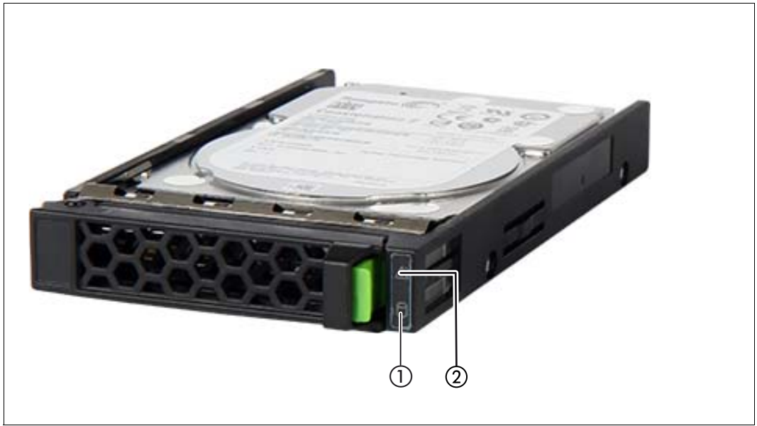
Figure 3: Indicators on a hot-plug HDD module
