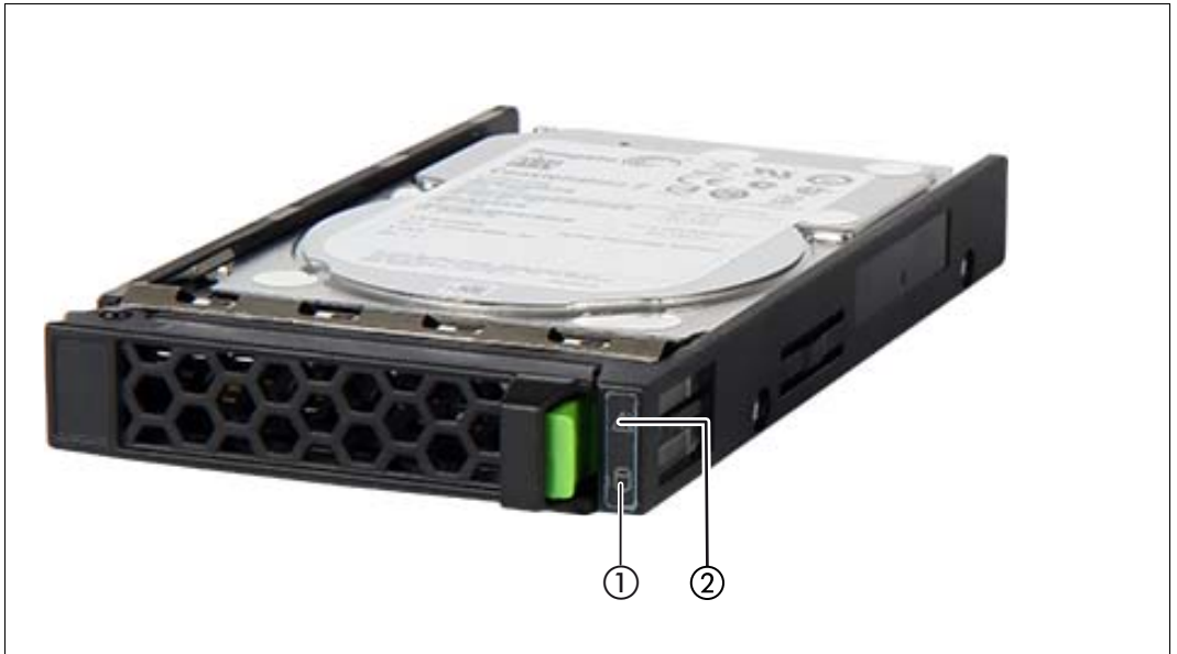
Figure 3: Indicators on a hot-plug HDD module
