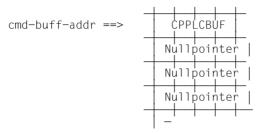
This field CPPLCBUF contains the address of the command buffer. The command buffer to which the address in field CPPLCBUF points must commence on a full word boundary and have exactly the same structure as for a TSO command processor.
