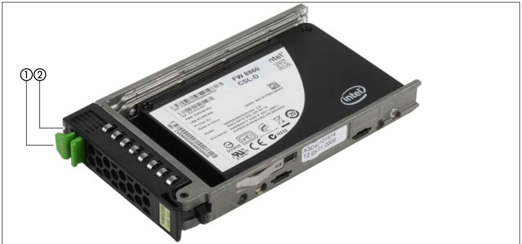
Figure 4: Indicators on the SSD drives
