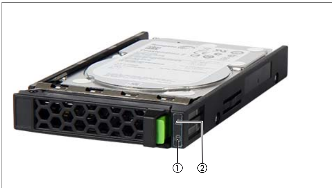
Figure 3: Indicators on a hot-plug HDD module
