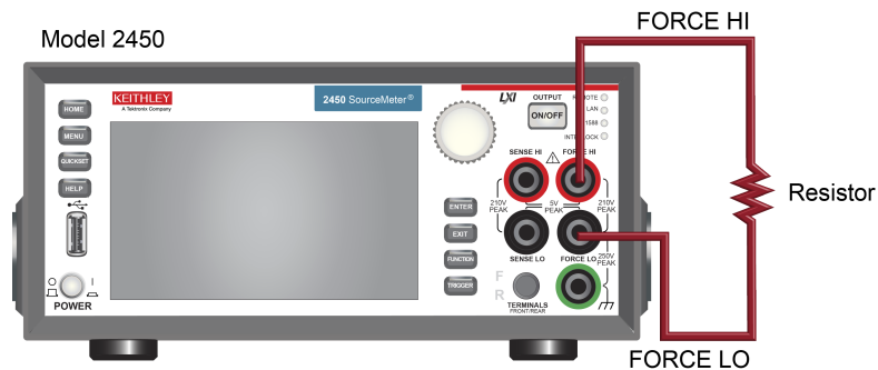
Figure 19: Model 2450 2-wire front-panel connections
