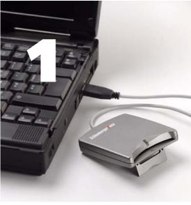
advantage of the smart card handling capabilities integrated in Microsoft Windows operating systems (the Personal Computer/Smart Card, or PC/SC, architecture).
