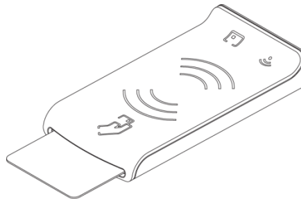
Figure 6 – The contactless smart card is put near or over the Prox-DU landing zone
