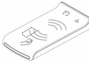
Figure 12 – The contact SIM/SAM card is inserted into the Prox-SU connector
