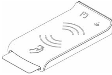
Figure 10 – The contact smart card is fully inserted into the Prox-DU slot
