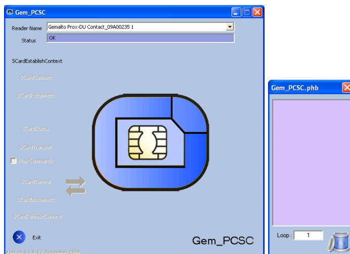
Figure 38 – Gem_PCSC window after “SCardReleaseContext”
