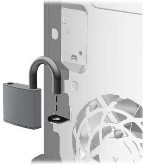
Figure 2-33 Installation d'un cadenas
