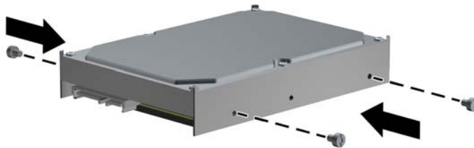
Figure 2-29 Installation des vis de guidage standard
