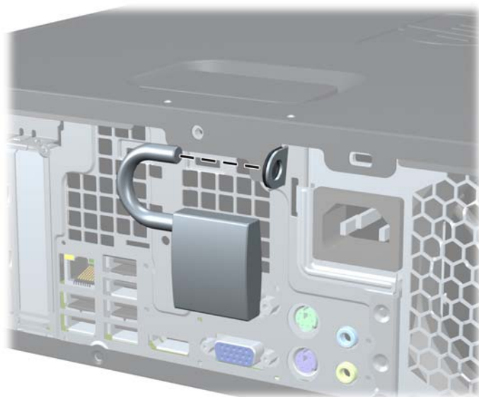
Figure C-2 Installation d'un cadenas
