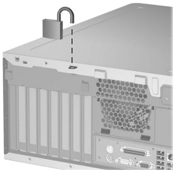
Figure C-2 Installation d'un cadenas
