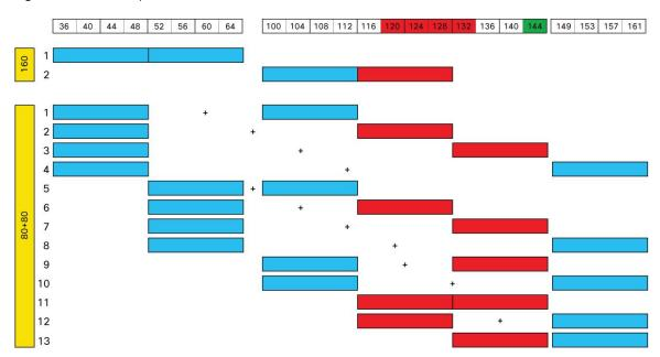
Figure 6. Channel Options for 160 MHz and 80+80 MHz
