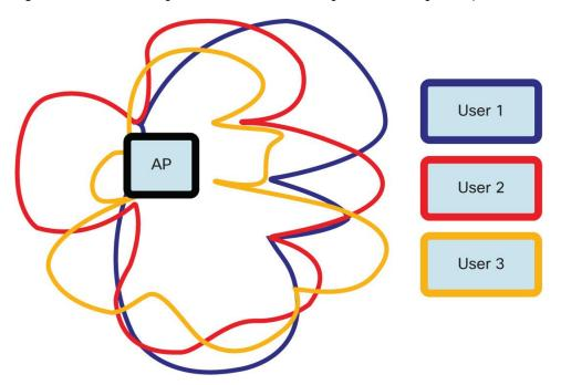
For all this to work properly, especially the deep nulls, the AP has to know the wireless channel from itself to all of the users very accurately. And since the channel changes over time, the AP has to keep measuring the channel, which adds overhead. Some APs might use the higher-overhead 802.11ac sounding protocol only, but the greatest benefit of MU-MIMO comes if the AP can minimize the number of explicit sounding exchanges, such as with the ClientLink mechanisms.
