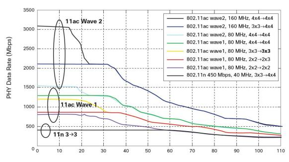
Figure 7. Simulation of Rate at Range for 802.11ac
