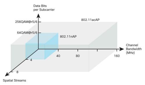
Figure 1. How 802.11ac Accelerates 802.11n
