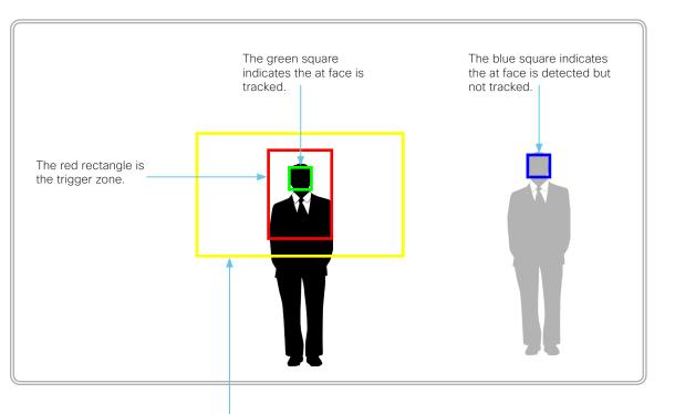
The yellow rectangle is the cropped image that follows the presenter. The yellow rectangle is not visible until a person steps into the trigger zone and is being tracked.
