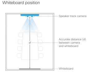
The whiteboard must be placed across the room from the camera, as shown in the illustration.
