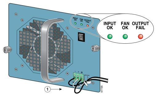
Figure 4-13 Connecting DC-Input Power to a Cisco 7304 Router
