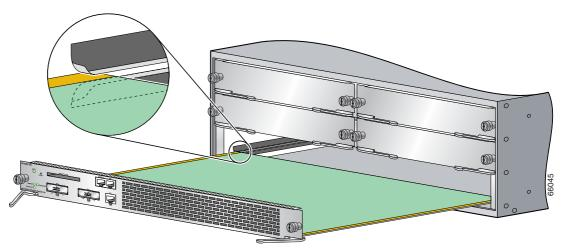
**Step 4** Position the locking levers at a 45-degree angle *before* installing the network services engine (see Figure 4-5).
