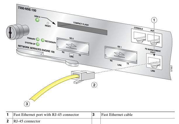
Figure 4-12 Attaching the Fast Ethernet Management Port 10/100 Cable
