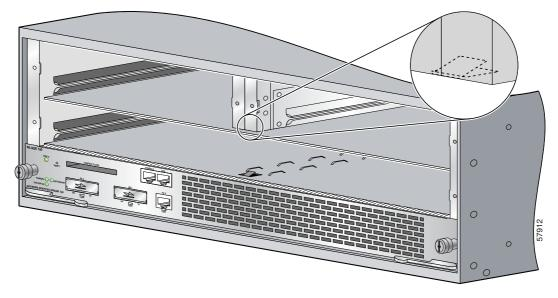
To remove the slot divider from the router, complete the following steps:
