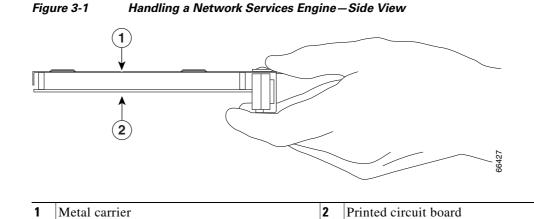
Although the metal carrier helps to protect the printed circuit boards from ESD, wear a preventive antistatic strap whenever handling a network services engine. Ensure that the strap makes good skin contact and connect the strap's clip to an unpainted chassis surface to channel unwanted ESD voltages safely to ground.
