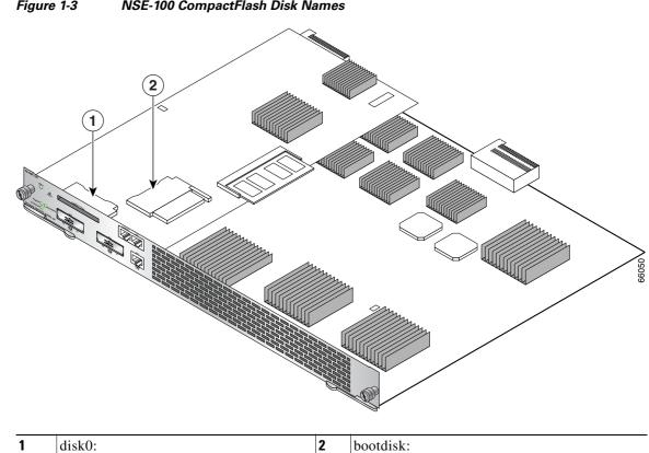
Figure 1-3 NSE-100 CompactFlash Disk Names
