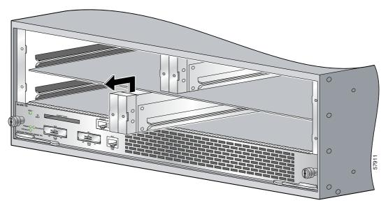
**Step 2** Slide the slot divider from the router (Figure 4-4).
