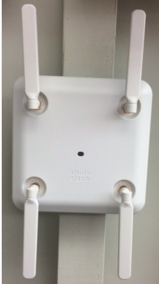
Figure 20: Avoid wall mounting units with internal antennas
