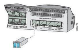
Step 5 If the module has a bale-clasp latch, close it to lock the SFP module in place.
