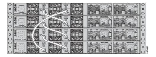
Figure 2-2 shows a recommended configuration when the switches are mounted side-by-side. Use the 1-meter and the 3-meter StackWise cables to connect the switches. This configuration provides redundant connections.
