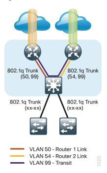
The distribution switch handles all access layer routing, with VLANs trunked to access switches. No HSRP is required when the design includes a distribution layer. A full distribution and access layer design is shown in the following figure.
