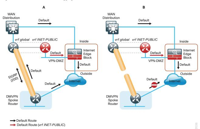
This configuration is referred to as *FVRF*, because the Internet is contained in a VRF. FVRF is sometimes referred to as *Front Side VRF*. The alternative to this design is Inside VRF (IVRF), where the internal network is in a VRF on the VPN hub and the Internet remains in the global VRF. This method is not documented in this guide.
