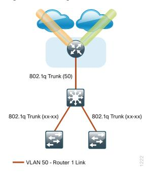
Figure 28 - IWAN dual router remote-site: Connection to distribution layer
