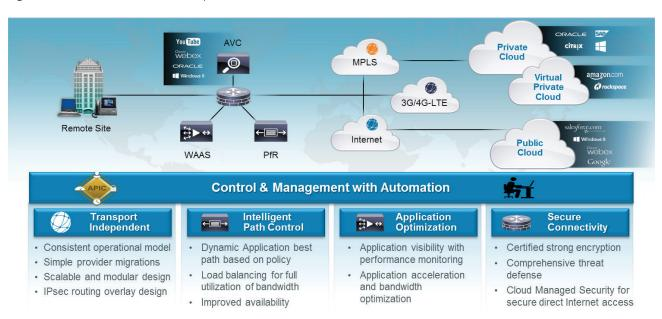
Figure 1 - Cisco IWAN solution components
