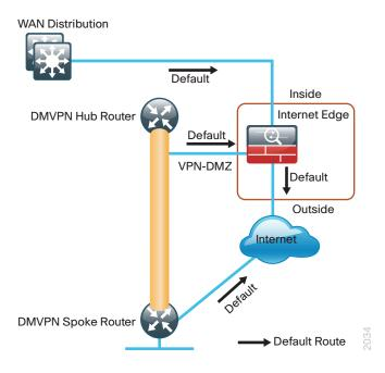
If you need to extend the internal network and the same default routing options that are available to internal users, you must advertise a default route to the VPN hub router. For details, see section A in the following figure.
