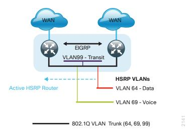
Enhanced object tracking (EOT) provides a consistent methodology for various router and switching features to conditionally modify their operation based on information objects available within other processes. The objects that can be tracked include interface line protocol, IP route reachability, and IP SLA reachability, as well as several others.
