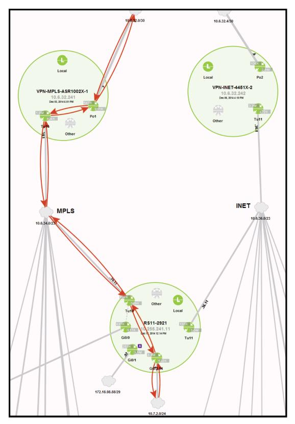
**Step 3:** After introducing loss into the MPLS path, verify that the protected traffic class is moved to the backup INET path by using the **show domain [name] master traffic-classes dscp** command.
