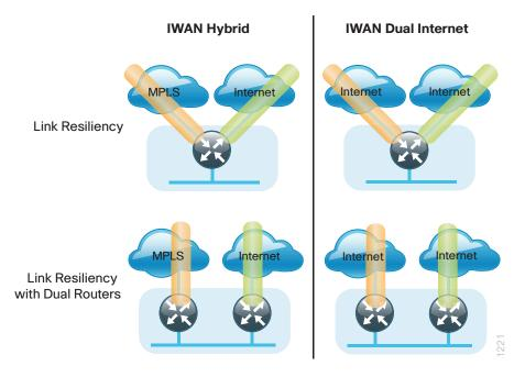
The remote-site designs include single or dual WAN edge routers. The remote-site routers are DMVPN spokes to the primary site hubs.
