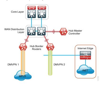
Figure 32 - IWAN hybrid design model: PfR branch locations
