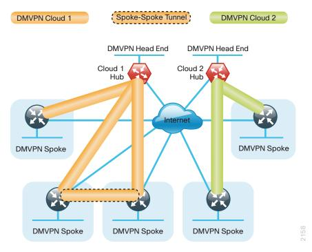
One of the key benefits of the DMVPN solution is that the spoke routers can use dynamically assigned addresses, often using DHCP from an Internet provider. The spoke routers can leverage an Internet default route for reachability to the hub routers and also other spoke addresses.
