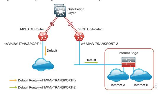
Figure 17 - IWAN dual Internet design model: FVRF default routing
