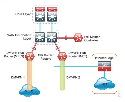
Figure 12 - Cisco Performance Routing: Remote site options
