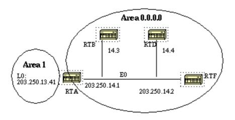
RTA, RTB, RTD, and RTF share a common segment (E0) in area 0.0.0.0. The following are the configs of RTA and RTF. RTB and RTD should have a similar configuration to RTF and will not be included.
