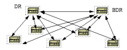
In the above diagram, all routers share a common multi-access segment. Due to the exchange of Hello packets, one router is elected DR and another is elected BDR. Each router on the segment (which already became a neighbor) will try to establish an adjacency with the DR and BDR.
