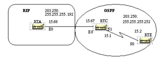
In the above diagram, RTE is running OSPF and RTA is running RIP. RTC is doing the redistribution between the two protocols. The problem is that the class C network 203.250.15.0 is variably subnetted, it has two different masks 255.255.255.252 and 255.255.255.192. Let us look at the configuration and the routing tables of RTE and RTA:
