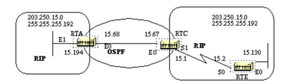
To illustrate, suppose RTA, RTC, and RTE are running RIP. RTC and RTA are also running OSPF. Both RTC and RTA are doing redistribution between RIP and OSPF. Let us assume that you do not want the RIP coming from RTE to be injected into the OSPF domain so you put a passive interface for RIP on E0 of RTC. However, you have allowed the RIP coming from RTA to be injected into OSPF. Here is the outcome:
