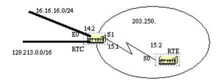
Suppose we added two static routes pointing to E0 on RTC: 16.16.16.0 255.255.255.0 (the /24 notation indicates a 24 bit mask starting from the far left) and 128.213.0.0 255.255.0.0. The following shows the different behaviors when different parameters are used in the **redistribute** command on RTC:
