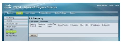
You cannot make any changes in the PSI Frequency table and can only view the available frequency plans stored in the receiver. The following is a list of the various columns:
