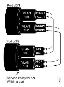
The following configuration file shows how to perform ingress and egress policing per VLAN using the policy-map P31\_QOS applied to port Gigabit Ethernet 3/1:
