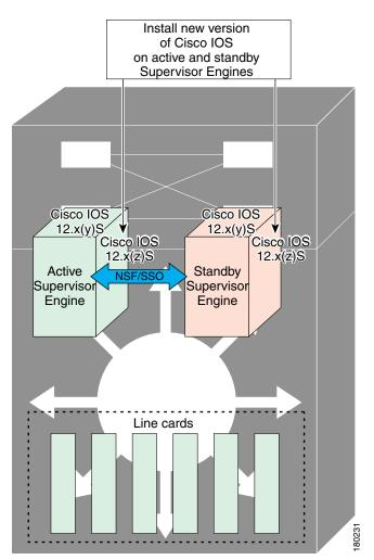
After you have copied the Cisco IOS software to both file systems, load the new version of Cisco IOS software onto the standby supervisor engine (see Figure 5).
