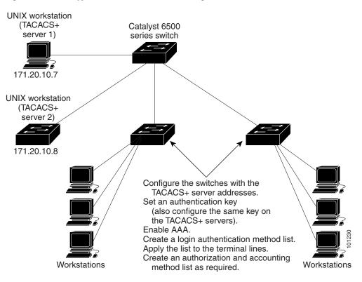
Figure 3-4 Typical TACACS+ Network Configuration
