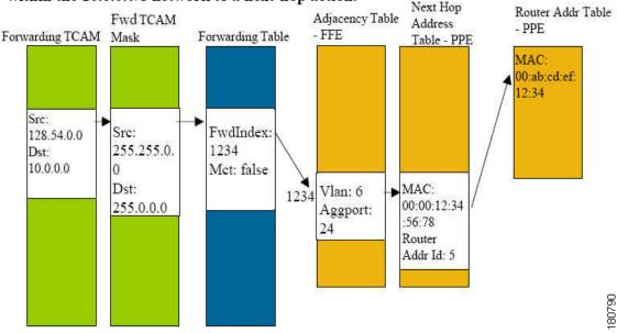
Figure 49-13 illustrates special adjacency entries created in the FIB.
