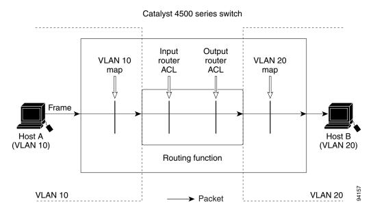
Figure 37-6 Applying ACLs on Routed Packets
