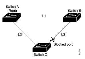
Figure 18-4 BackboneFast Before Indirect Link Failure
