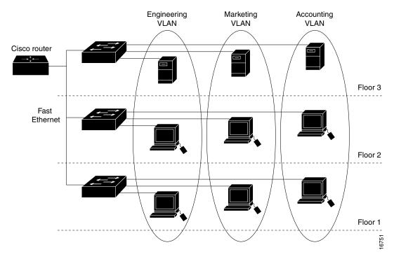
VLANs are often associated with IP subnetworks. For example, all of the end stations in a particular IP subnet belong to the same VLAN. Traffic between VLANs must be routed. You must assign LAN interface VLAN membership on an interface-by-interface basis (this is known as interface-based or static VLAN membership).
