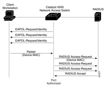
Figure 32-4 Message Exchange during MAC Authentication Bypass
