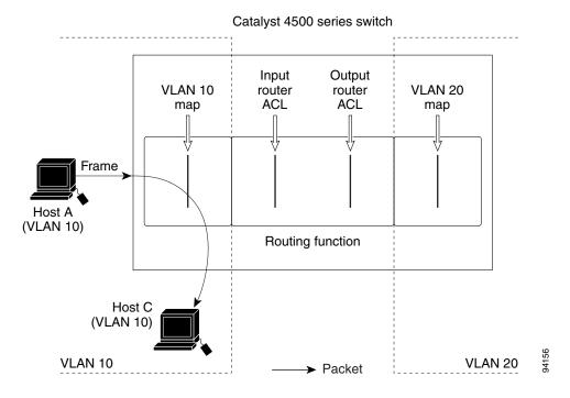
Figure 37-5 Applying ACLs on Switched Packets
