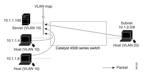
This procedure configures ACLs with VLAN maps to deny access to a server on another VLAN. The VLAN map SERVER 1\_ACL denies access to hosts in subnet 10.1.2.0/8, host 10.1.1.4, and host 10.1.1.8. Then it permits all other IP traffic. In Step 3, VLAN map SERVER1 is applied to VLAN 10.
