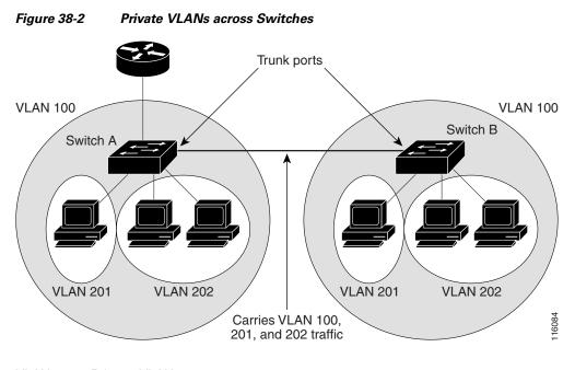
VLAN 100 = Primary VLAN VLAN 201 = Secondary isolated VLAN VLAN 202 = Secondary community VLAN
