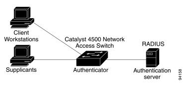
• Client—The workstation that requests access to the LAN, and responds to requests from the switch. The workstation must be running 802.1X-compliant client software.
