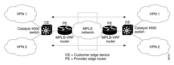
Figure 29-1 Catalyst 4500 Series Switches Acting as Multiple Virtual CEs
