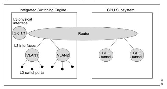
Figure 26-2 Hardware and Software Switching Components
