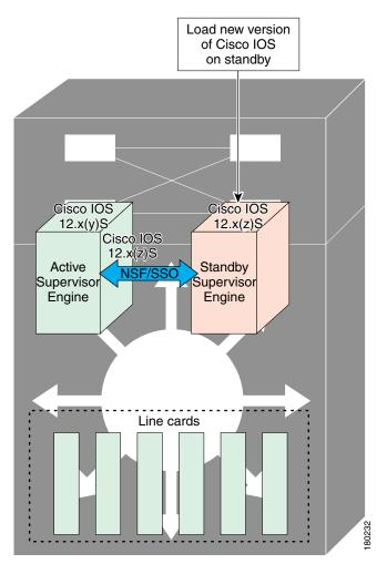
After a switchover (NSF/SSO, not RPR), the standby supervisor engine takes over as the new active supervisor engine (see Figure 6).
