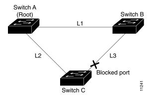
If Switch C detects a link failure on the currently active link L2 on the root port (a direct link failure), UplinkFast unblocks the blocked port on Switch C and transitions it to the forwarding state without going through the listening and learning states, as shown in Figure 18-3. This switchover takes approximately one to five seconds.
