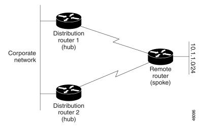
Figure 5 shows a simple dual-homed remote with one remote router and two distribution routers. Both distribution routers maintain routes to the corporate network and stub network 10.1.1.0/24.
