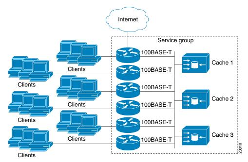
Figure 47-1 Cisco Content Engine Network Configuration Using WCCP
