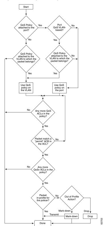
Figure 30-4 Policing and Marking Flowchart
