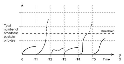
The broadcast suppression threshold numbers and the time interval combination make the broadcast suppression algorithm work with different levels of granularity. A higher threshold allows more broadcast packets to pass through.
