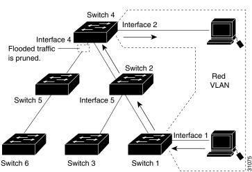
Figure 13-3 Flooding Traffic with VTP Pruning
