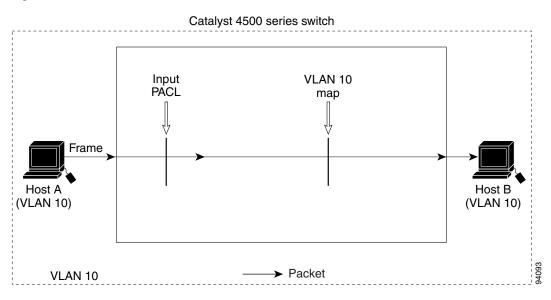
If the interface access group mode is prefer port, then only the input PACL is applied on the ingress traffic from Host A. If the mode is prefer vlan, then only the VACL is applied to the ingress traffic from Host A. If the mode is merge, the input PACL is first applied to the ingress traffic from Host A, and the VACL is applied on the traffic.
