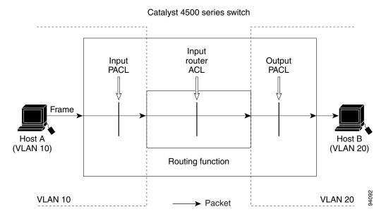
If the interface access group mode is prefer port, then only the input PACL is applied on the ingress traffic from Host A. If the mode is prefer vlan, then only the input Router ACL is applied to ingress traffic from Host A that requires routing. If the mode is merge, then the input PACL is first applied to the ingress traffic from Host A, and the input Router ACL is applied on the traffic that requires routing.
