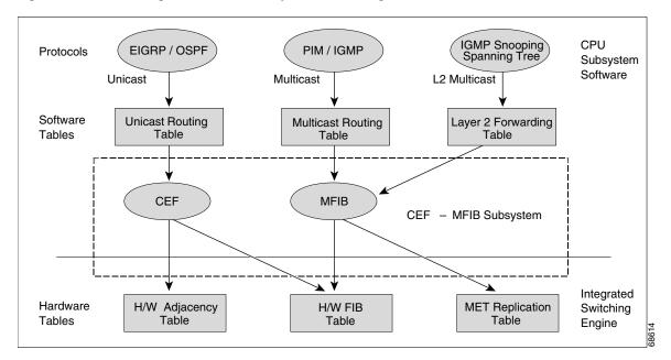
Like the CEF unicast routes, the MFIB routes are Layer 3 and must be merged with the appropriate Layer 2 information. The following example shows an MFIB route:
