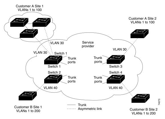
Figure 21-5 Layer 2 Network Topology without Proper Convergence
