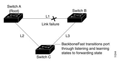
Figure 18-5 BackboneFast after Indirect Link Failure
