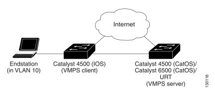
Figure 13-6 Dynamic Port VLAN Membership Configuration
