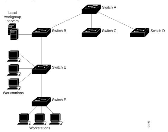
Figure 4-1 Typical NTP Network Configuration
