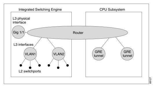
Figure 27-5 Hardware and Software Forwarding Components
