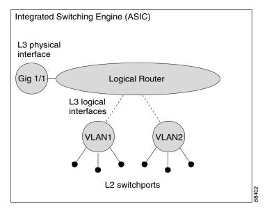
Figure 26-1 Logical L2/L3 Switch Components
