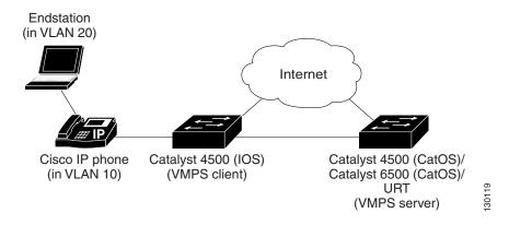
In the following procedure, the Catalyst 4000 and Catalyst 6000 series switches (running CatOS) are the VMPS servers. Use this procedure to configure the Catalyst 4500 series switch clients in the network:
