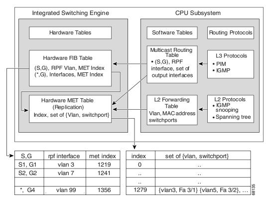
Figure 27-4 IP Multicast Tables and Protocols
