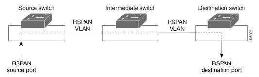
SPAN and RSPAN do not affect the switching of network traffic on source ports or source VLANs; a copy of the packets received or sent by the sources is sent to the destination. Except for traffic that is required for the SPAN or RSPAN session, by default, destination ports do not receive or forward traffic.
