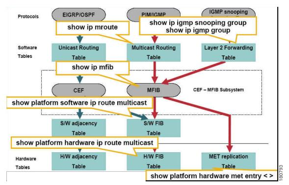
Figure 49-3 Multicast Programming Flow
