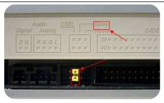
4. From your main board, find out the 40-pin Secondary IDE interface cable. Then connect them to your CD-R/RW. Please do notice that the color edge of the IDE cable must be aligned with PIN 1 of the IDE controller.
