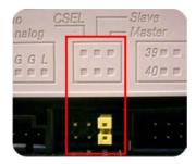
Note: Installing jumper pins besides the ones for device configuration settings may be the cause of damage or abnormal drive operation.
