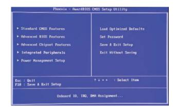
Now you can move the cursor by using direction keys on the keyboard. Move the cursor to the option item "Load Optimized Defaults" and press "Enter" button.
