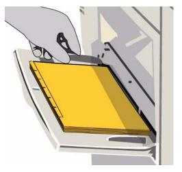
**Note:** It is important to ensure that the machine knows which tray contains the tab stock as the print driver will select the tray by stock type and size. Always select the correct Size, Color and Type after loading the stock in the tray.
