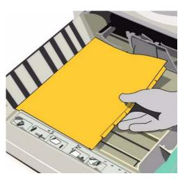
2 Adjust the paper guides to touch the side and back of the stack of tabs.
