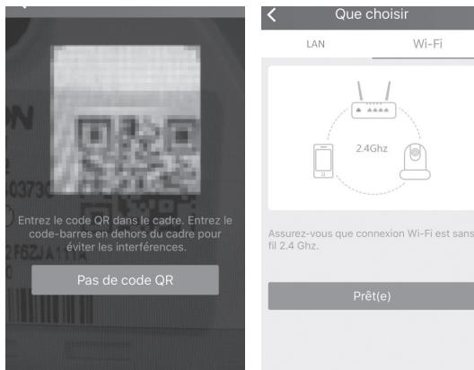
Once the code has been read, your smartphone or tablet will ask you to choose between Lan and Wifi. Select Wi-Fi and press "**prêt(e)**" (ready), please enter the key to the WiFi network you are connected to, to be able to transmit it to the camera.
